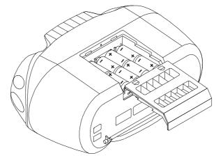
3.) Replace the battery compartment door.
